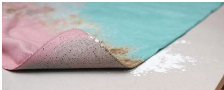
Fig. 6.3.4: Water and moisture contamination on fabric
