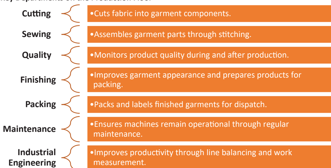
Fig. 1.1.8: Key Departments on the Production Floor
