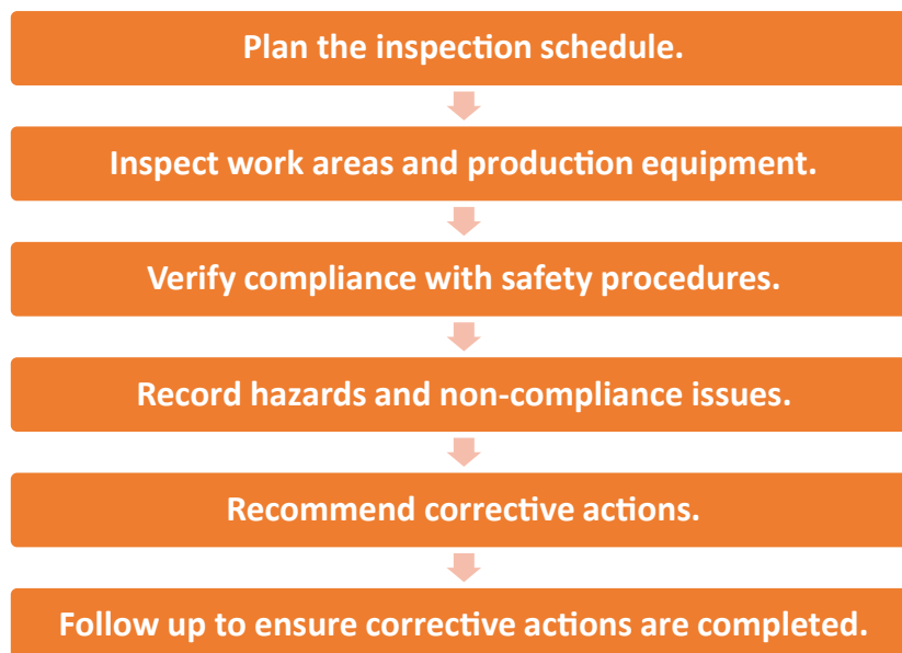
Fig. 6.1.2: Steps in a Safety Inspection
