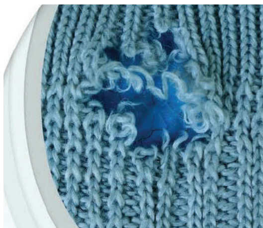
Fig. 2.1.11: Knitted garment construction defects
