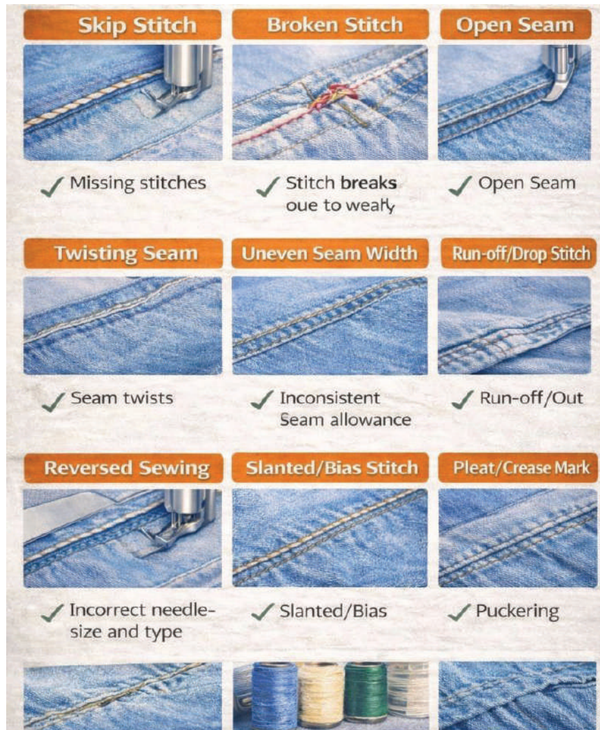
Fig. 2.1.12: Tailored and structured garment defects
