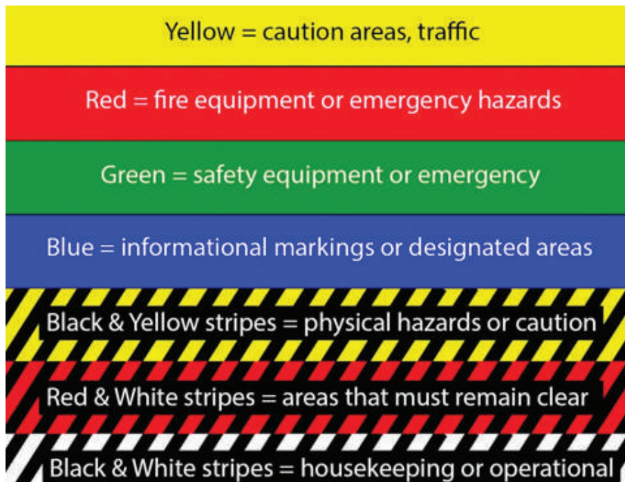
Fig. 6.2.7: Colour-coded floor marking
