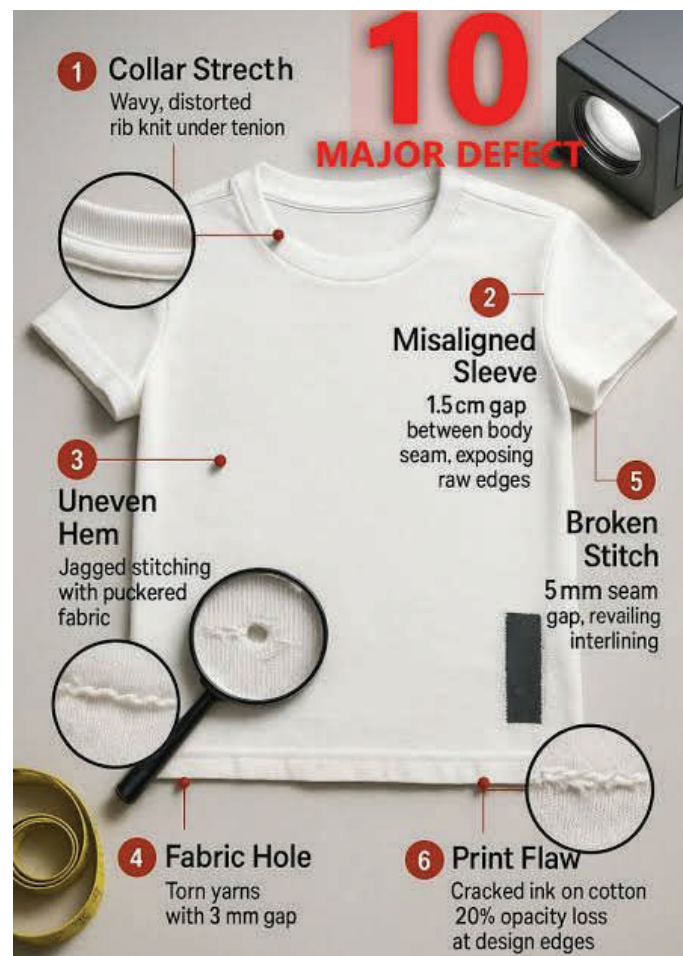
Fig. 2.1.8: Garment construction defects
