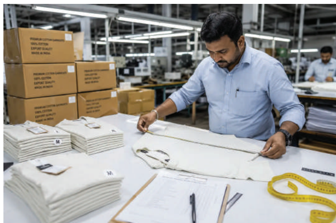
Fig. 1.1.12: Apparel quality analyst in AQL inspection
