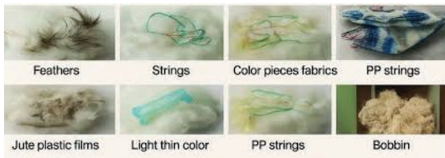
Fig. 8.3.2.: Dust and fibre contamination in fabric
