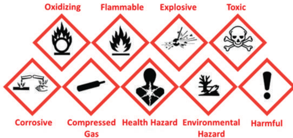
Fig. 8.1.6: Chemical hazard identifiers
