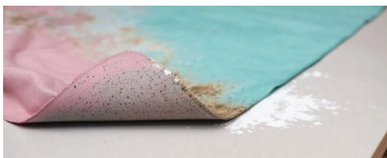
Fig. 8.3.4: Water and moisture contamination on fabric
