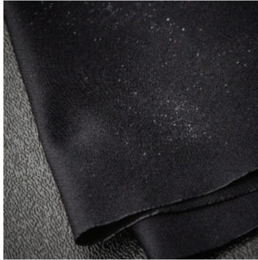
Fig. 8.3.5: Foreign material contamination on fabric
