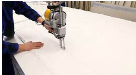
Fig. 3.2.7: Straight knife cutting
