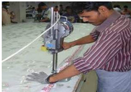
Fig. 3.2.8: Band knife cutting technique
