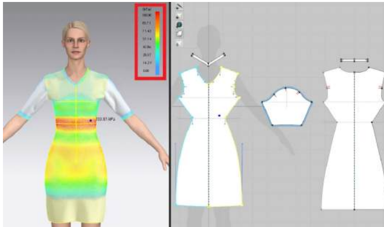
Fig. 3.1.23: Digitising pattern using CAD (Computer-Aided Design) software
