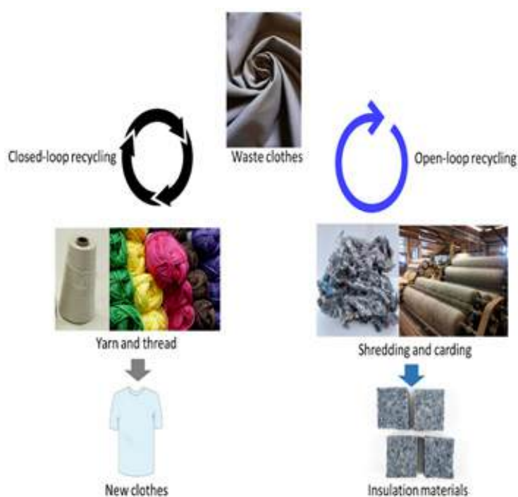
Fig. 9.2.3: Closed-loop and open-loop mechanical recycling of textiles
