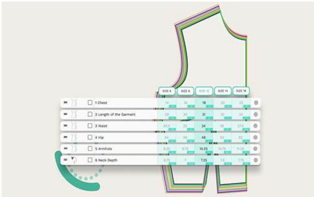
Fig. 3.1.21: Pattern grading using specific software
