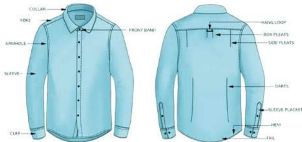
Fig. 3.1.4: Components of a shirt
