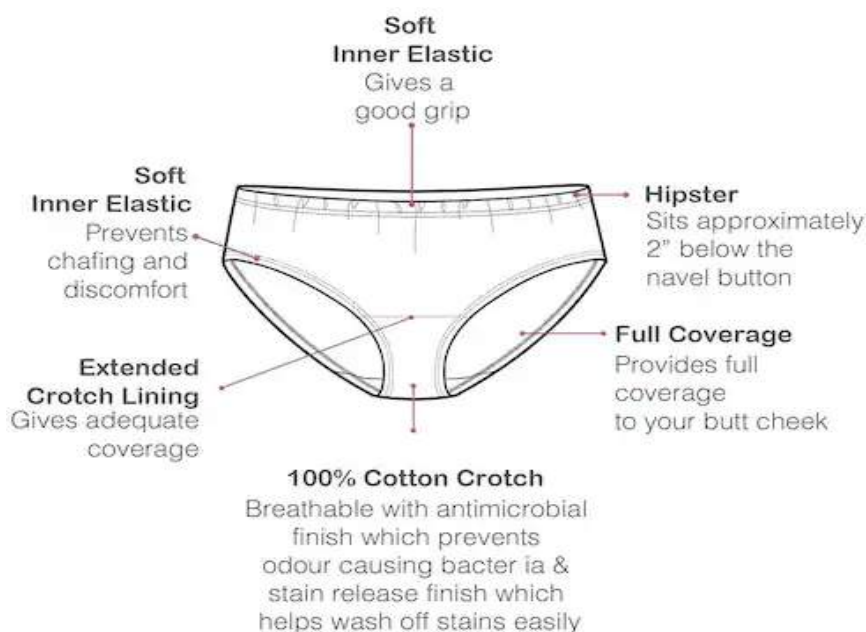
Fig. 3.1.10: Components of an undergarment
