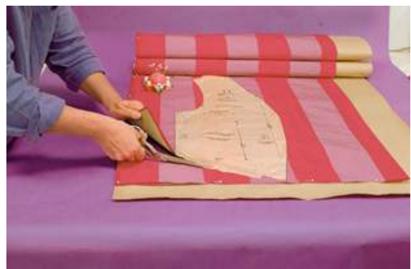
Fig. 3.1.14: Secure edges with clamps or weights during cutting
