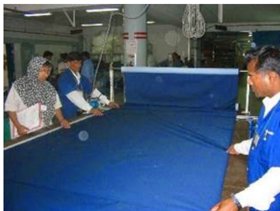
Fig. 3.1.4: Checking fabric faults
