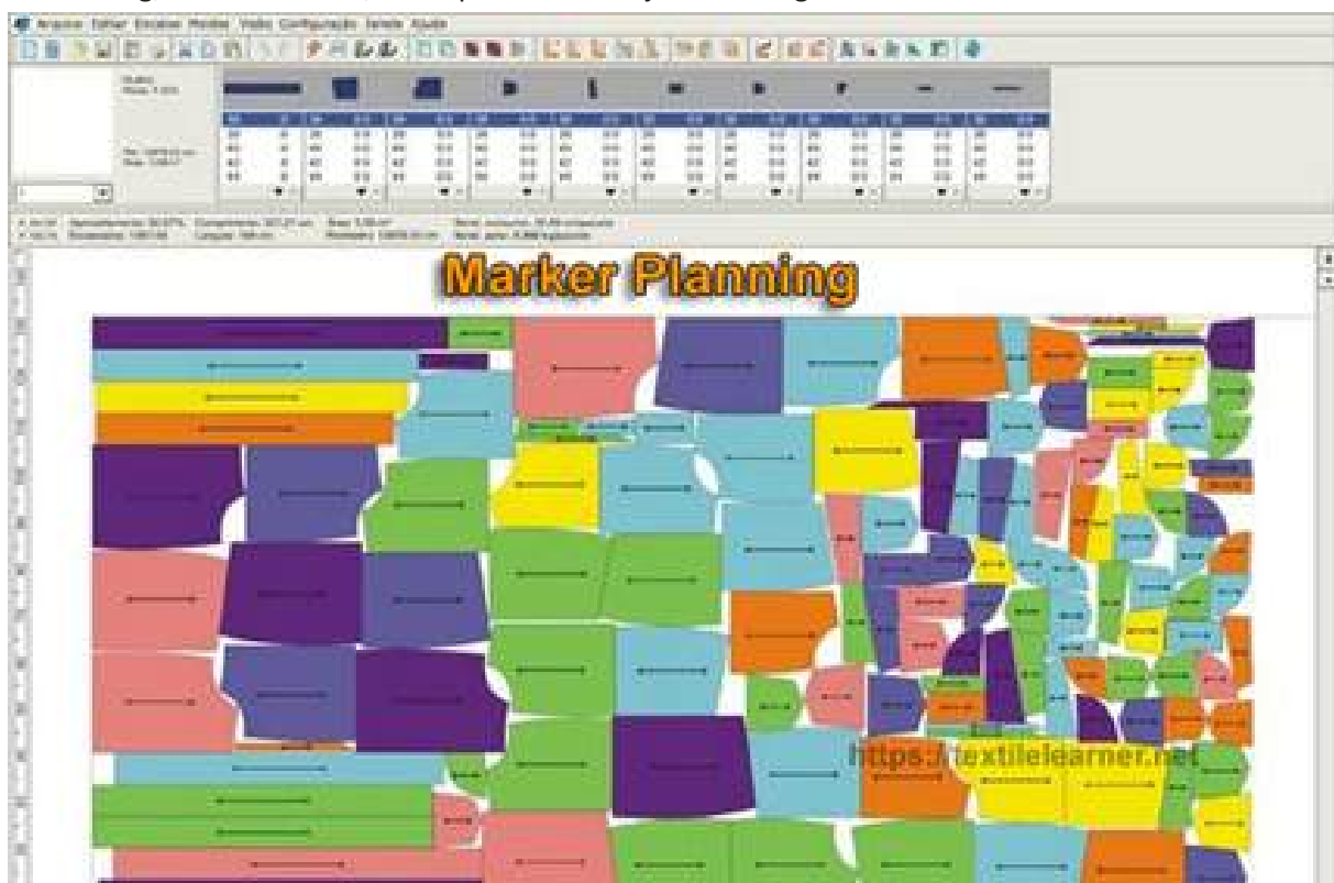
Fig. 4.1.2: Marker making on software
