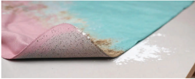
Fig. 7.3.4: Water and moisture contamination on fabric
