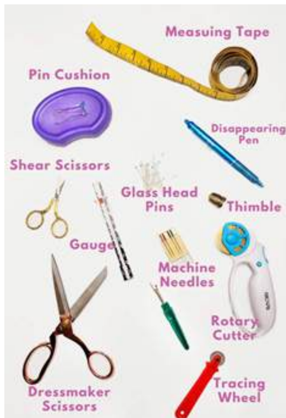
Fig. 4.3.1: Safe Usage of Stitching Tools and Equipment
