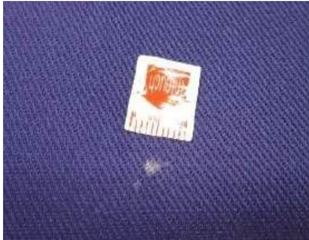
Fig. 2.1.39: Dirt/stains on fabric
