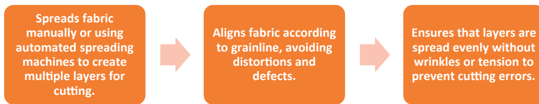
Fig. 1.1.17: Steps when laying the fabric
