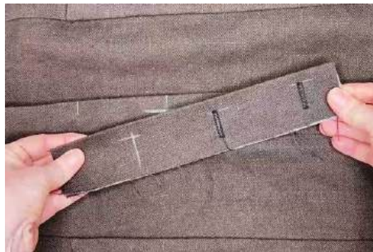
Fig. 5.1.23: Placement of buttonholes
