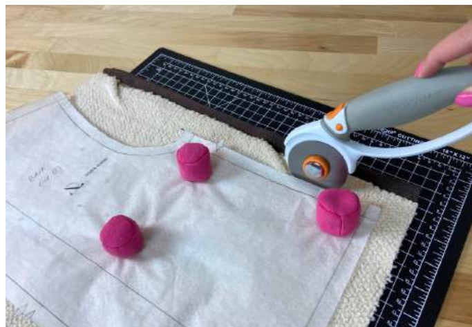
Fig. 5.1.5: Rotary cutter to cut fabric precisely
