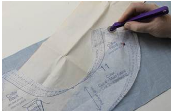
Fig. 4.1.6: Tracing wheel and carbon paper
