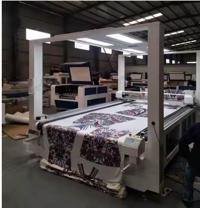
Fig. 5.2.17: Laser-cutting of fabric
