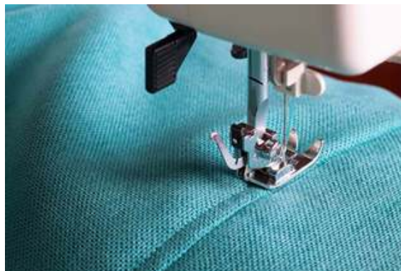
Fig. 7.1.10: French Seam Stitching Technique
