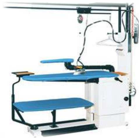
Fig. 4.1.14: Pressing and finishing equipment
