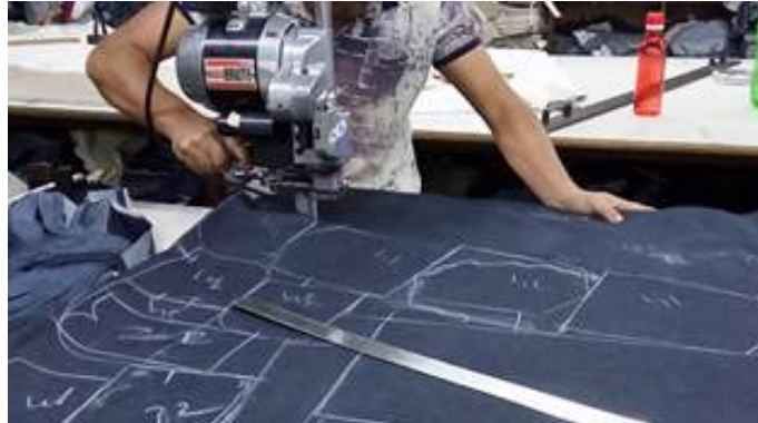
Fig. 7.1.2: Straight Knife Cutting
