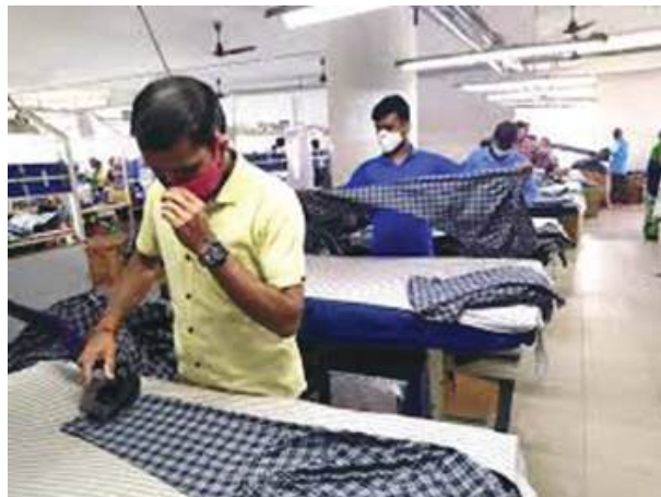
Fig. 3.3.1: Preventative measures during pressing
