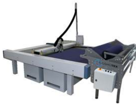
Fig. 9.2.6: Cradle feed spreading machine
