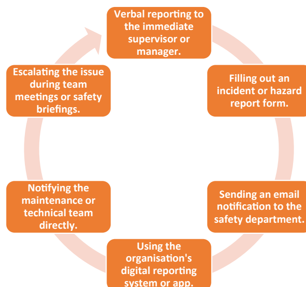
Fig. 11.2.2: Way to report unsafe equipment and other dangerous occurrences to concerned personnel
