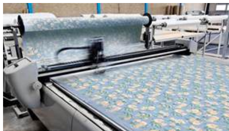
Fig. 8.2.7: AI detector for defects
