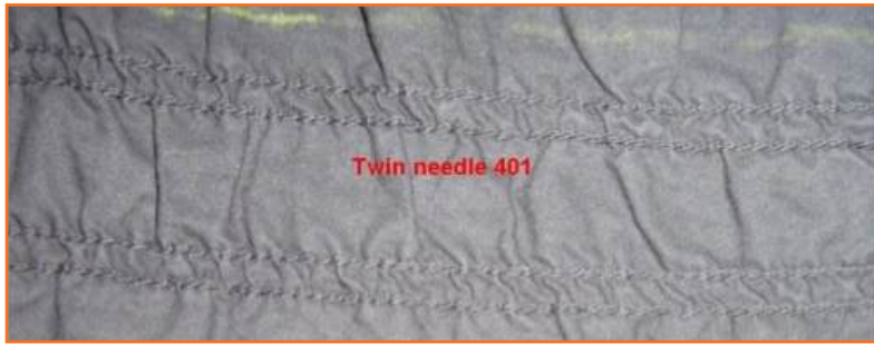
Fig 3.2.9: : Shrinkage pucker occurs during the
