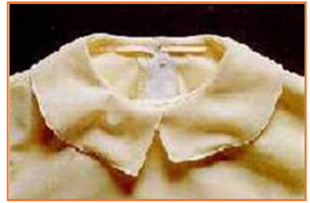
Fig 3.2.17(c): Interlining shrinking
