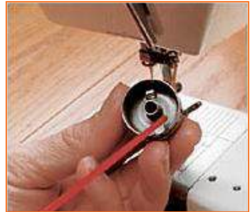
Fig 4.1.1: Cleaning the bobbin and case
