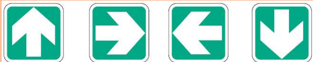
Fig.5.1.17: Signs for emergency exits
